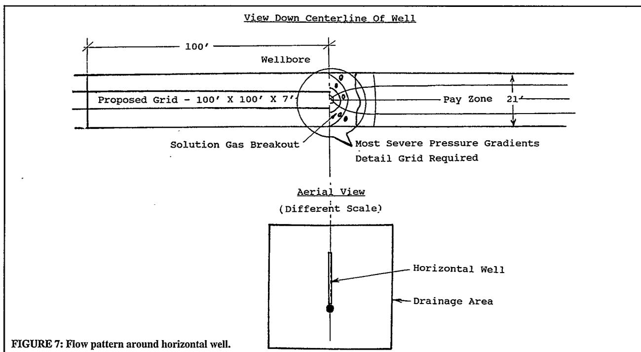
FIGURE 7: Flow pattern around horizontal well.
