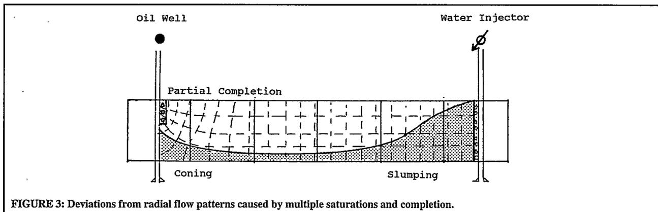
FIGURE 3: Deviations from radial flow patterns caused by multiple saturations and completion.
