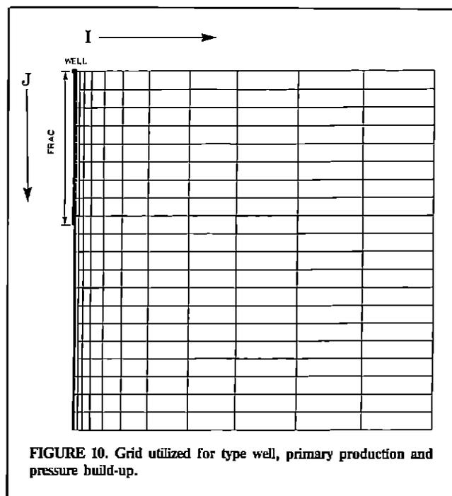
FIGURE 10. Grid utilized for type well, primary production and pressure build-up.
