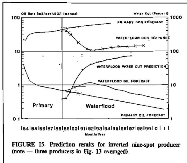
**FIGURE 15. Prediction results for inverted nine-spot producer (note — three producers in Fig. 13 averaged).**
