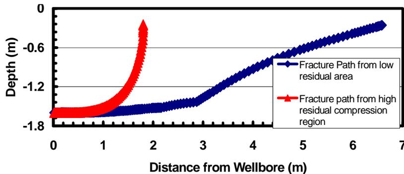
Figure 6 FRACANAL Fracture Shapes – Horizontal Frac
