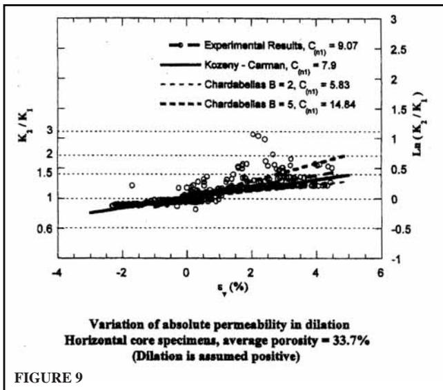
is given in Figures 8<sup>(8)</sup> and 9<sup>(9)</sup>. At volumetric strains of 4%, roughly corresponding to the peak strengths of the samples, the vertical permeabilities increased by 100%. Some specimens had an increase in absolute permeability of one order of magnitude during the test. Permeability increases were attributed to dilation and shearing. Restated, pore volume increase and widened flow paths increased pore connectivity.
