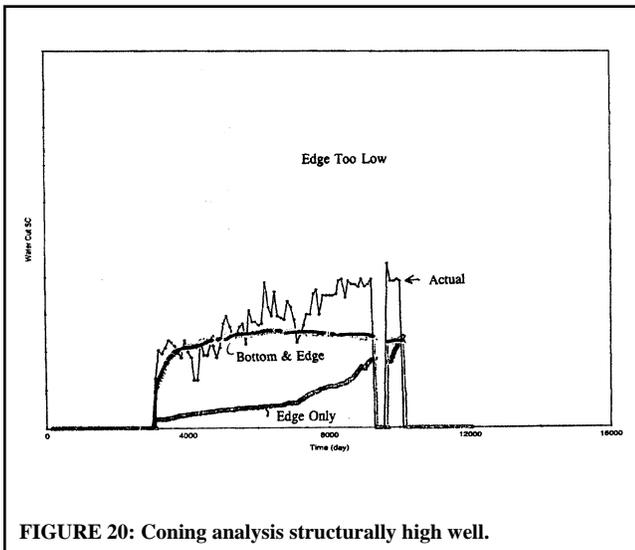
FIGURE 20: Coning analysis structurally high well.
