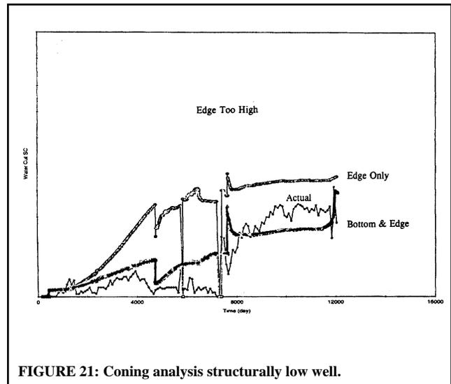
FIGURE 21: Coning analysis structurally low well.
