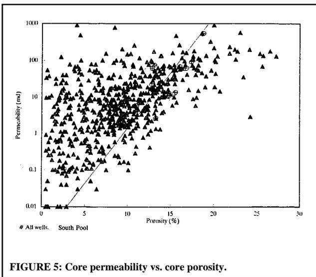
FIGURE 5: Core permeability vs. core porosity.
