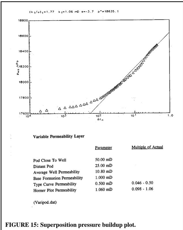
FIGURE 15: Superposition pressure buildup plot.
