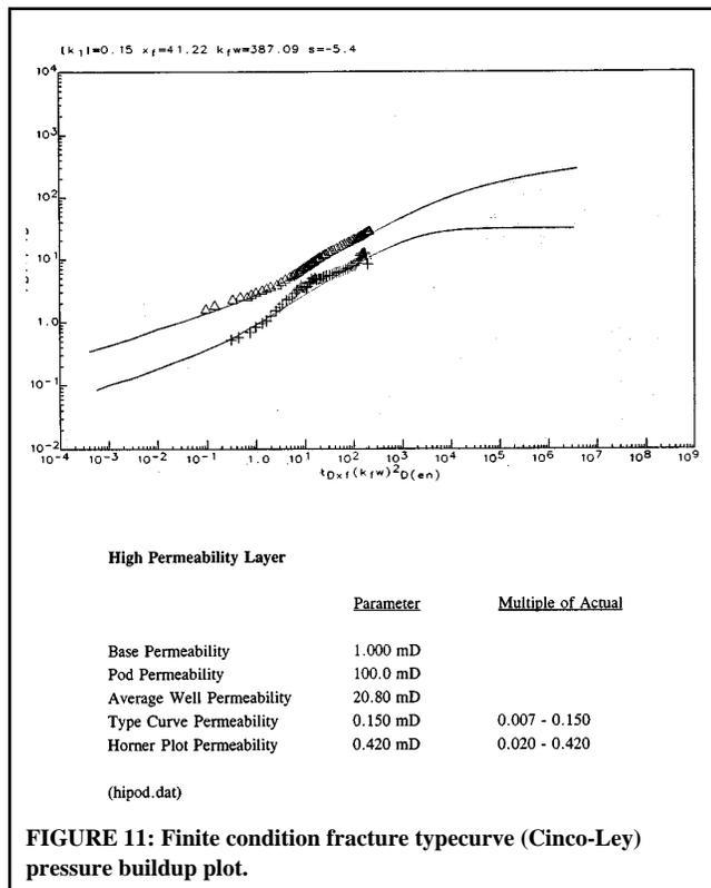
FIGURE 11: Finite condition fracture typecurve (Cinco-Ley) pressure buildup plot.
