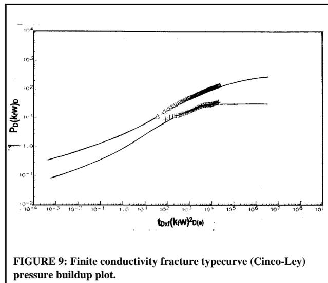
FIGURE 9: Finite conductivity fracture typecurve (Cinco-Ley) pressure buildup plot.
