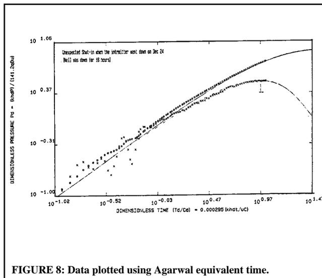
FIGURE 8: Data plotted using Agarwal equivalent time.
