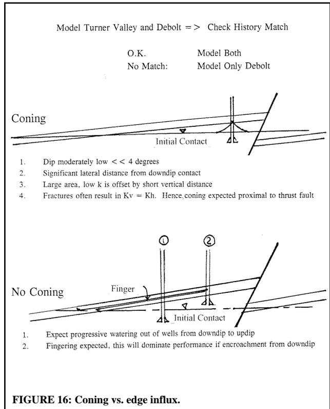
FIGURE 16: Coning vs. edge influx.
