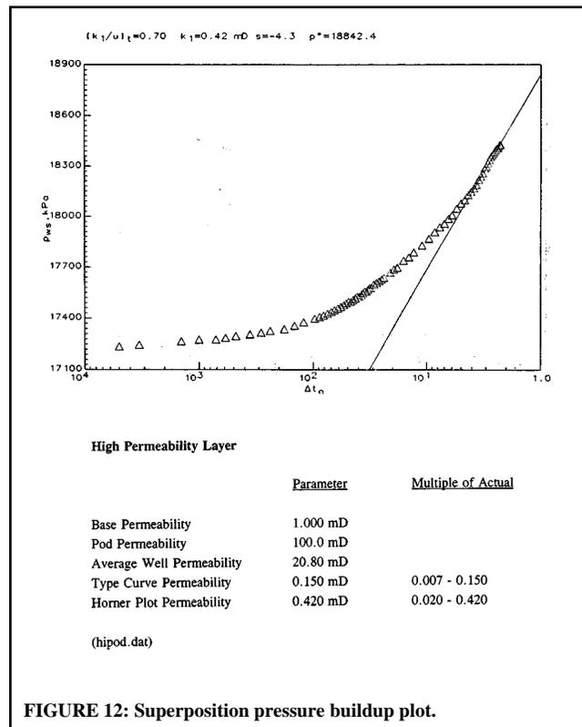
FIGURE 12: Superposition pressure buildup plot.
