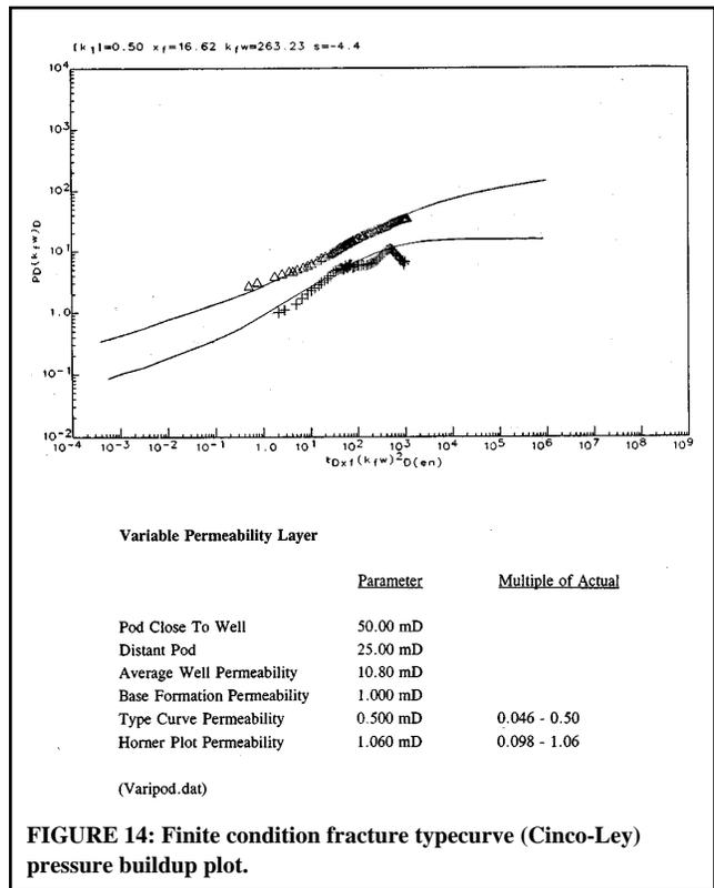
FIGURE 14: Finite condition fracture typecurve (Cinco-Ley) pressure buildup plot.
